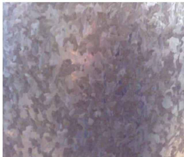
Figure 2 : Surface aspect of the hot-dip galvanized steel
